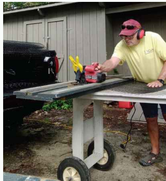
Photos left to right: 1. Spring 2023 Float Sale at Deltaville Maritime Museum. Drone photo courtesy of Kent Eanes. 2. High speed wire cutter saves time and labor when we are building hundreds of cages. Photo courtesy of Judy Spain.
