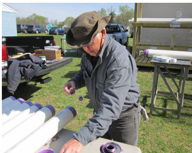
TOGA volunteer Bob Dunkle paints primer on a PVC pipe for a Taylor float at a Float Build Thursday in preparation for the Fall '25 Float and Spat Sale at Camp Kekoka
