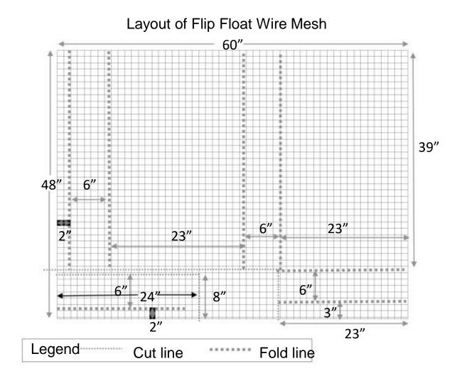
The diagram shows the cut lines and fold (or bend) lines for the 5 ft. by 4 ft. piece of wire mesh.
