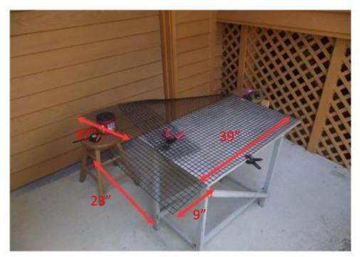
Cut out lower left panel leaving the dimensions shown. Be sure to remove all nubs in the finish pieces (They can cut skin if not trimmed closely). The 23" by 9" panel left attached will become the bottom of the box. The 37" by 9" panel cut out will be further cut to become the lid.
