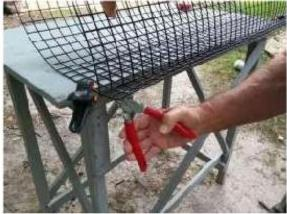
Now tighten the seam of the wire cylinder by firmly clamping 1/2" pig rings every 4 inches along the outside edge of the overlap. Then attach a few more pig rings to the inside edge of the overlap.
