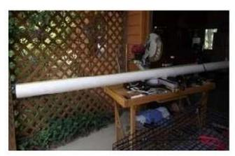
PVC drain or sewer pipe comes in 10 foot lengths. Cut one 33.5 inch piece for each Tidal Tumbler. None are required for a Rough Rider. You can cut the pipe with a compound miter saw, jigsaw, circular saw, or hand saw. Note that this is 4" diameter thin-wall drainpipe. It is cheaper and lighter than schedule 40 PVC pipe. The 4" end caps shown are sold in the same section of most building product stores.
