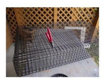
The pig rings along the back edge of the lid create a hinge.
