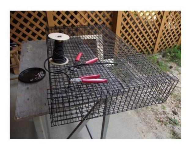
Cut a 23" length of bungee cord. Attach one end as shown with 2 pig rings.
