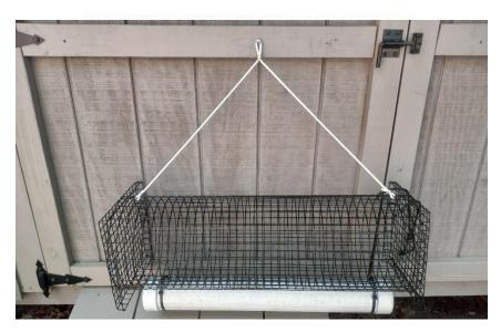
For the Tidal Tumbler only, attach the PVC tube along the overlap seam. Use a 24 inch cable tie at each end just inside of the end cap to secure the PVC tube to the wire cylinder. Cut off the excess cable tie once secured. Use a 5 foot piece of crab pot line to create a harness which is attached opposite from the PVC float. Use 2 pig rings for the loop at the apex and to attach each end.
