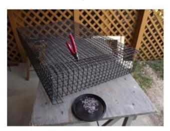
Pig ring all seams, roughly 5 to 6 in. apart. Note that the bottom seam and side seam are overlapped, and therefore reinforced.
