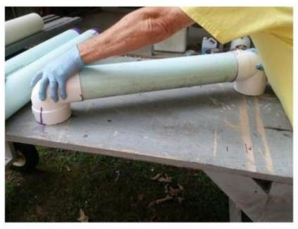
After priming and adding glue, insert the long tubes as shown.
