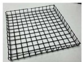
Fixed end piece bent one inch on all four sides
