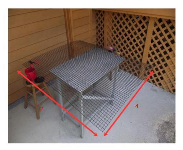
Start with a 5' length of wire mesh that is cut from a 4' wide roll. TOGA buys 16 gage vinyl-coated wire from Ocean Products Research in Diggs (Mathews), VA.
