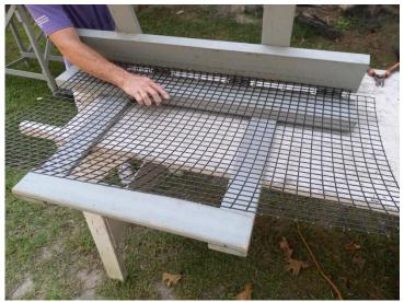
Starting on a long edge, bend the outer 2 rows of mesh into a triangular stiffener, as shown, using ~ 135 degree bends. Repeat on the opposite long edge.
