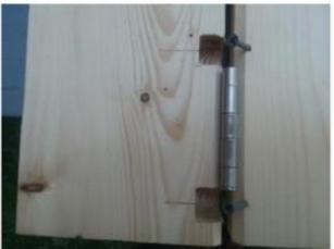
Place 3 inch door hinges between the screws as shown. I like to use 1.25 deck screws rather that the screws that come with the hinges.
