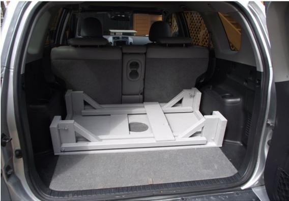
**Shucker on the Go-** For the volunteer party in March, we needed oyster shucking tables and suddenly realized they were hard to transport in cars. So I made a folding rig that fits in an average trunk. When folded, it's 40 in. long, 24 in. wide, and about 10 in. high. The hole in the middle is convenient for dumping your shells in a bucket. Also good for float building or general work. Comes painted.
