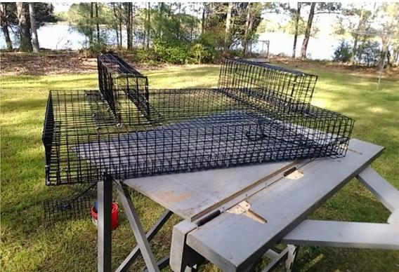
**Good Feet-** It turned out that our previous version of the bottom cage had bad feet that tended to rack or collapse under water. The new version has sturdy feet. We will replace your bottom cage feet at the October 3 Float Workshop, or by request. The photo shows the new configuration.
